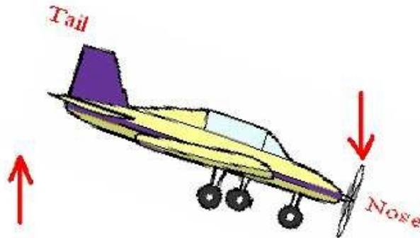
Case (iii): PROPELLER rotates in ANTICLOCKWISE direction when seen from rear end and Aeroplane turns towards LEFT
