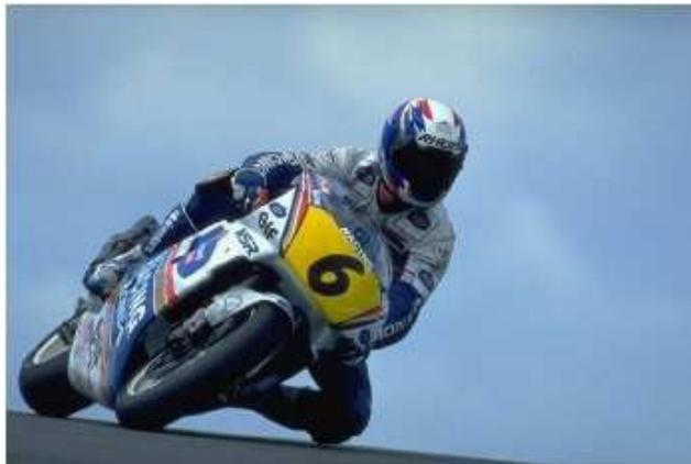
Fig shows a two wheeler vehicle taking **left turn** over a curved path. The vehicle is inclined to the vertical for equilibrium by an angle  $\theta$  known as angle of heel.
