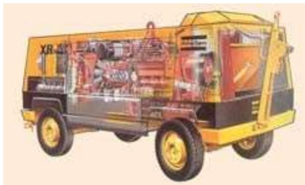
This industrial compressor uses compressed air to power heavy-duty construction tools. Compressors are used for jobs, such as breaking up concrete or paving, drilling, pile driving, sand-blasting and tunnelling. A compressor works on the same principle as a pump. A piston moves backwards and forwards inside a hollow cylinder, which compresses the air and forces it into a hollow chamber. A pipe or hose connected to the chamber channels the compressed air to the tools.
